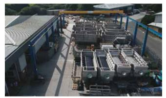
PYREG pyrolysis technology, whereby dewatered and (pre) dried sludges or screenings are pyrolysised and reduced to a valuable biosolid. At present, this biosolid end-product is used as an effective soil conditioner. But, it's not hard to imagine that microplastics that have been treated by the PYREG technology could then be incinerated, perhaps on a local site by site basis. Another sister company owns a very efficient and effective advance oxidation process (AOP) based on ozone and ultrasound.
